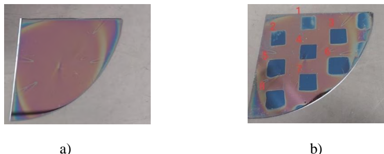
Fig. 1: Photograph of the contrast patterns of the homopolymer a) before and b) after exposure at 254nm and thermal treatment
